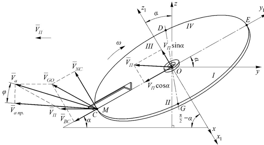
**Fig. 1. Equivalent system of fertiliser particle leaving the disc of the fertilizer-dispersing working organ considering the initial speed of the aggregate**
